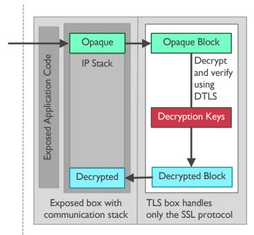
Initial keys provisioned by System Integrator. Messages decoded independent of stacks using mbed TLS in separate security context
