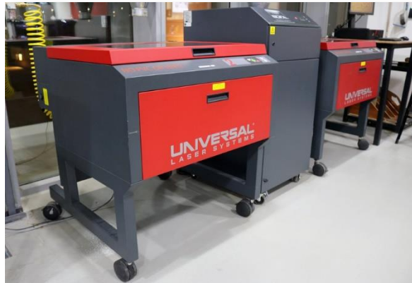
Laser cutting the above design into 6mm Acrylic sheet takes around 15 minutes with a low-power 60W CO 2 Laser Cutter.
