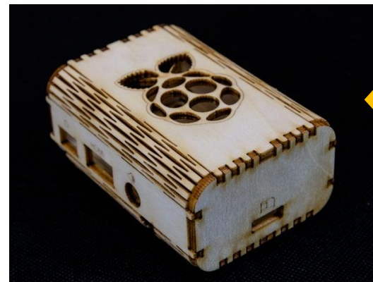
FlexiPi + Raspberry Pi case using Kerf patterning for bends by Iron Momo @ thingiverse.com .
